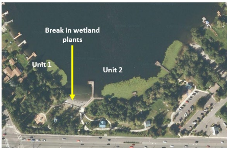
Figure 8. Break in lake fringe vegetation along a shoreline. The yellow arrow shows the absence of wetland plants along the shore that separates the wetlands into two units for rating.
