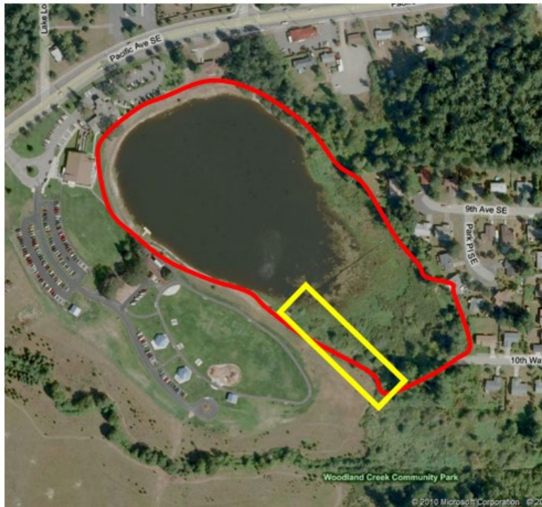
Figure 1. Footprint of the impact is the yellow rectangle, but the unit for rating is the entire wetland (red line).
