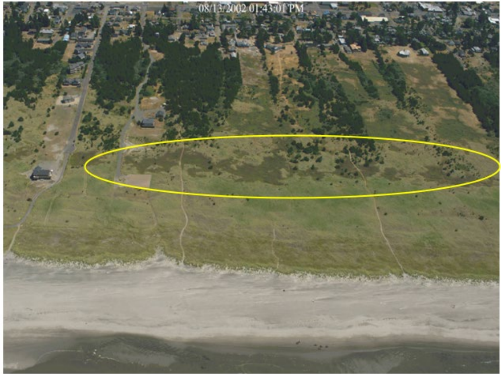
Figure 52. Intertidal mosaic that is larger than 1 ac. Individual wetland areas within the oval may be smaller than 1 ac, but they form a mosaic that is larger than 1 ac.
