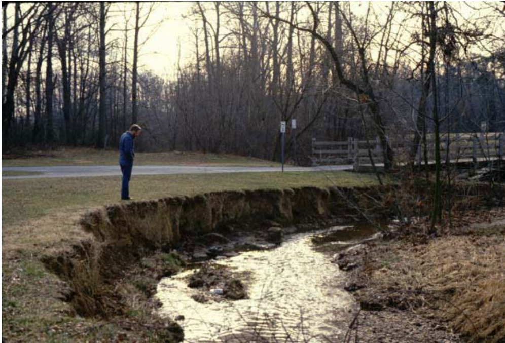
Figure 33. A stream in a watershed with approximately 20% impervious surface cover showing downcutting. You would answer YES to question R 5.1 for this stream.
