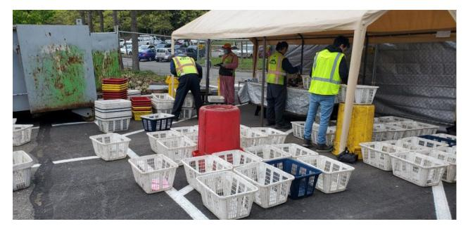
Figure 18. Sorting crew hand-sorting items into material classes.
