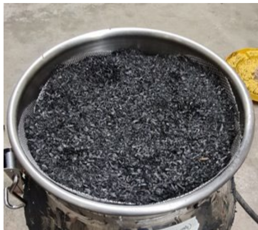
Figure 12: Biochar biofilter. Small wells are visible at the surface where air has flowed through preferentially after day 3
