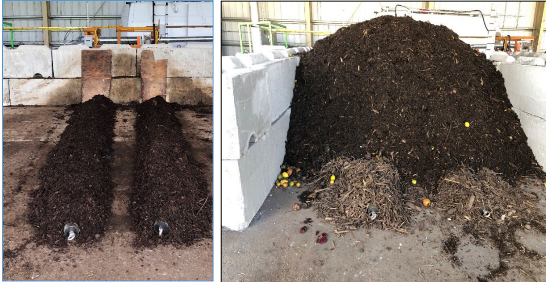
Figure 3: Photos of aeration plenum with compost covers covering aeration tubes (right photo) and a picture as pile is being built into the bunker.
