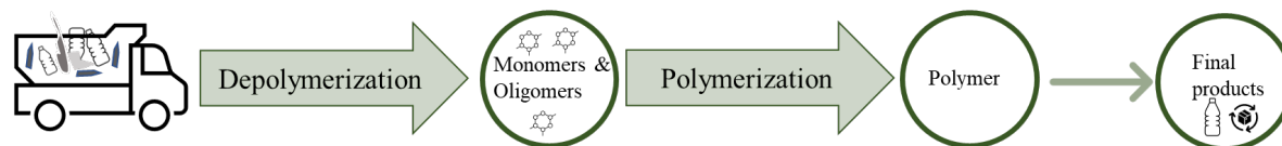
Figure 9. A scheme representing chemical depolymerization processes.
