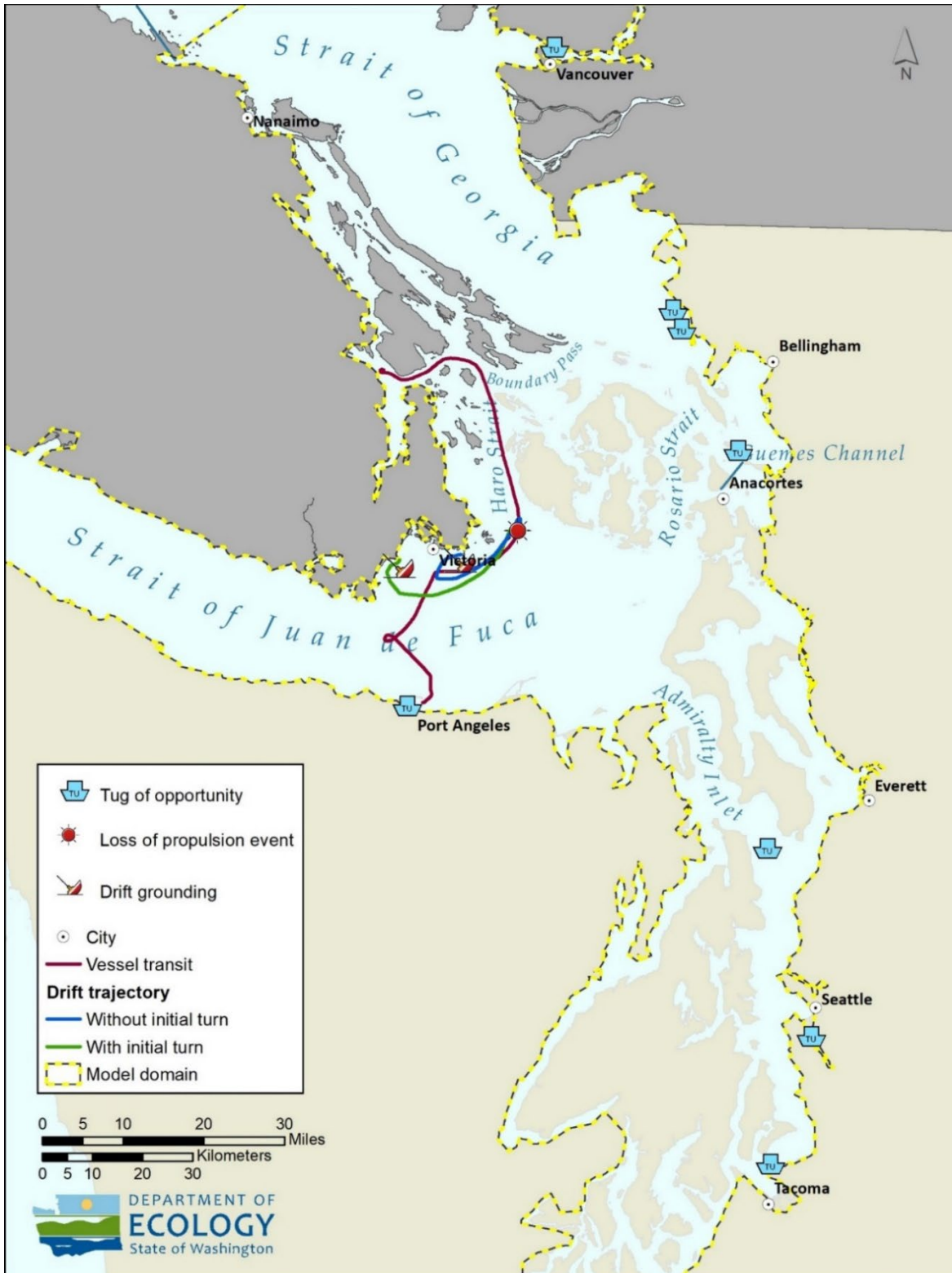
Figure B-10: Map showing tugs of opportunity when loss of propulsion occurs.
