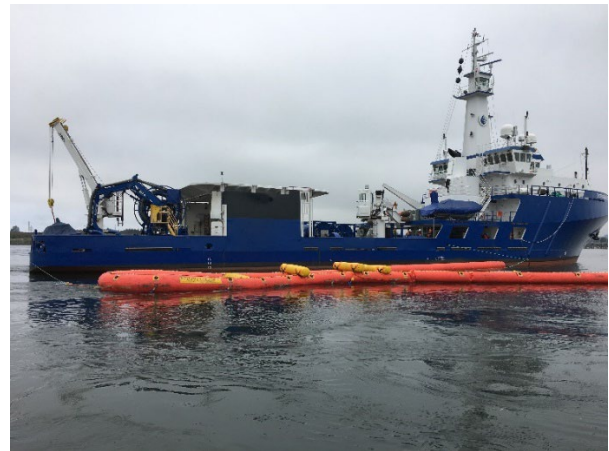
Figure 2. A deployment exercise to test oil spill response equipment.
