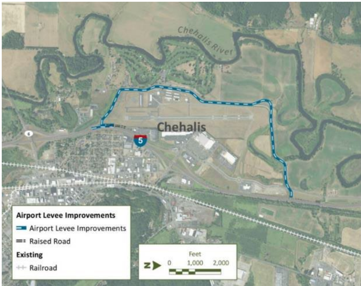
Figure 9. Map of the proposed raised levee and road near the Chehalis-Centralia Airport Source: FCZD, 2022.
