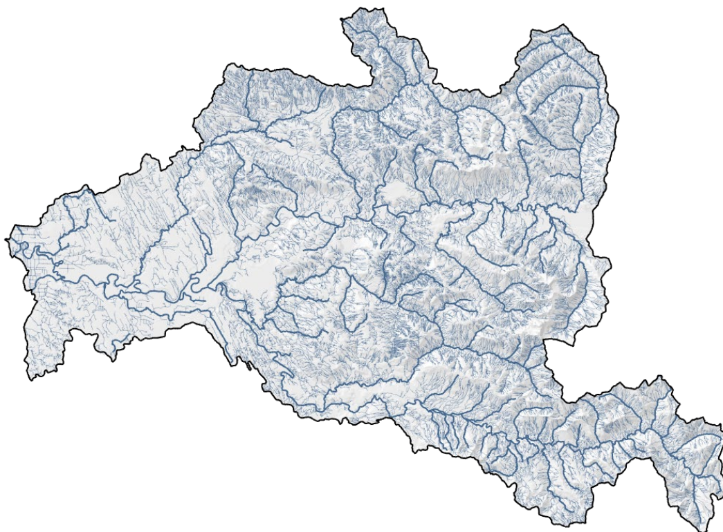
Figure 15. GNIS streams (thick lines) and non-GNIS streams (thin lines) from final EDH dataset in the Stillaguamish watershed.
