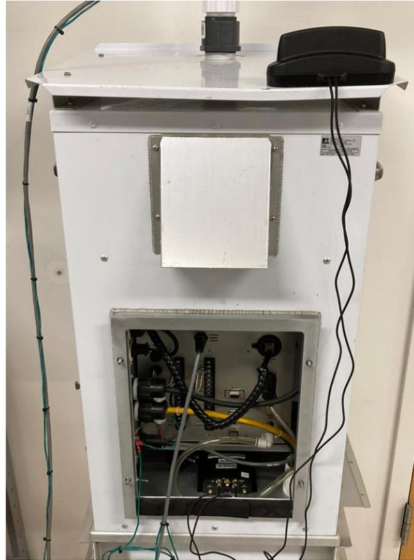
Figure 5-1: BAM 1022 stand-alone setup with cellular modem
