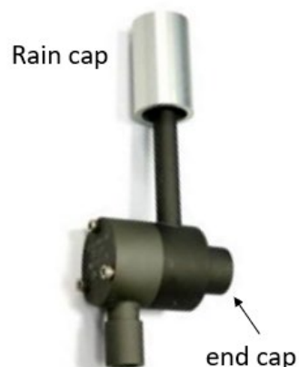
Figure 5-3: Inlet PM 2.5 cyclone
