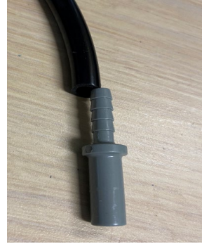
Figure 5-1: Spare line for easier leak and flow checks
