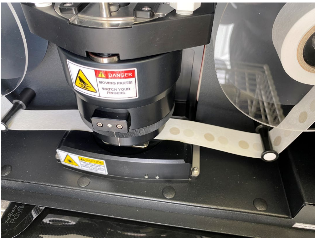
Figure 2-2: Dual spot collection on the Aethalometer filter tape
