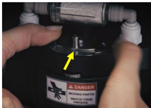
Figure 5-4: Lifting the optical chamber and locking mechanism
