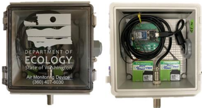
SensWA sensor device (6”x6”x4” and approximately 3 lb)
