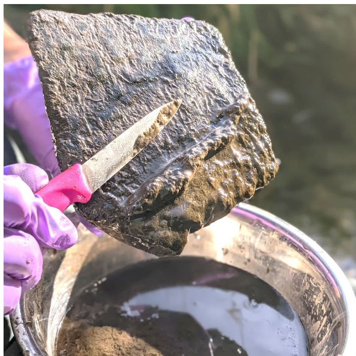
Figure 4. Biofilm scraped from a cobble during field sampling.
