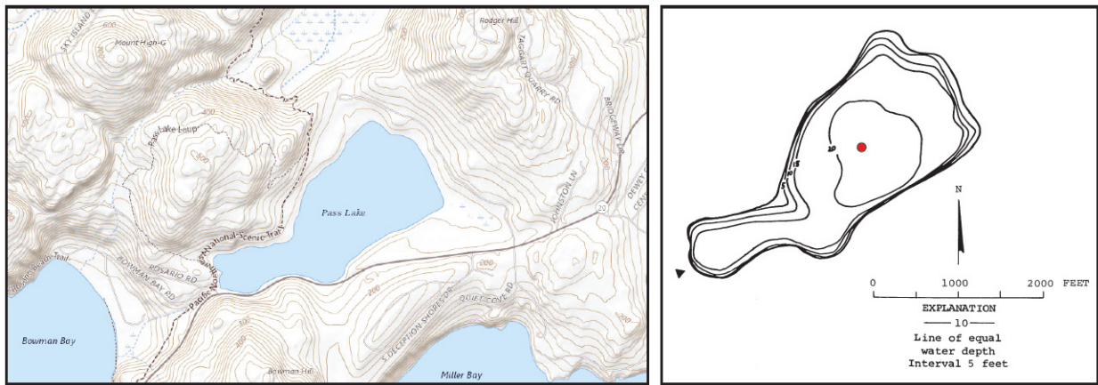
Figure 3. (left) Pass Lake watershed, (right) lake bathymetry and lake sediment core location (red dot).
