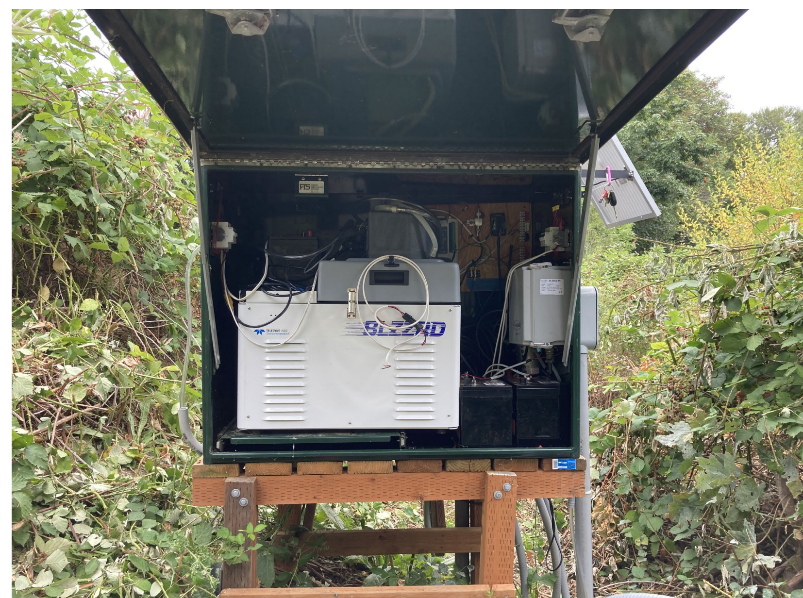
Figure 2. A refrigerated ISCO Sampler and Data Collection Platform in a telemetered station.
