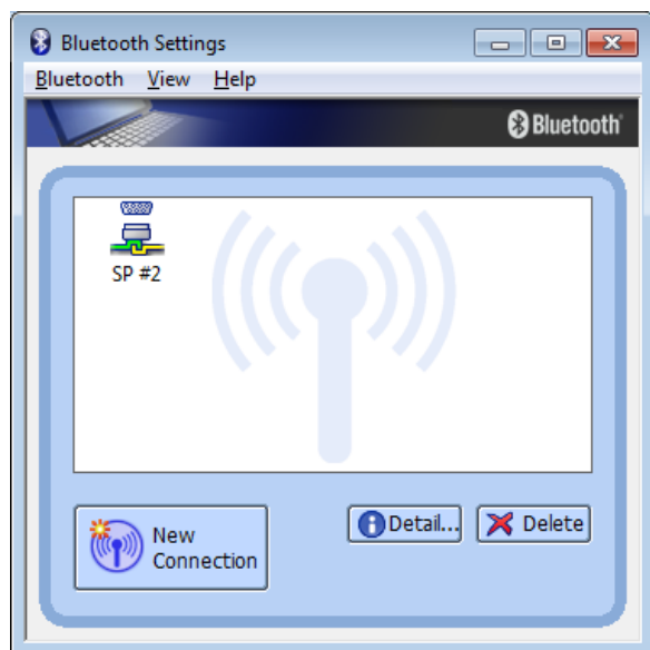
Figure A5. Bluetooth Manager screen showing Bluetooth connected icon (interlocking yellow and green bars).
