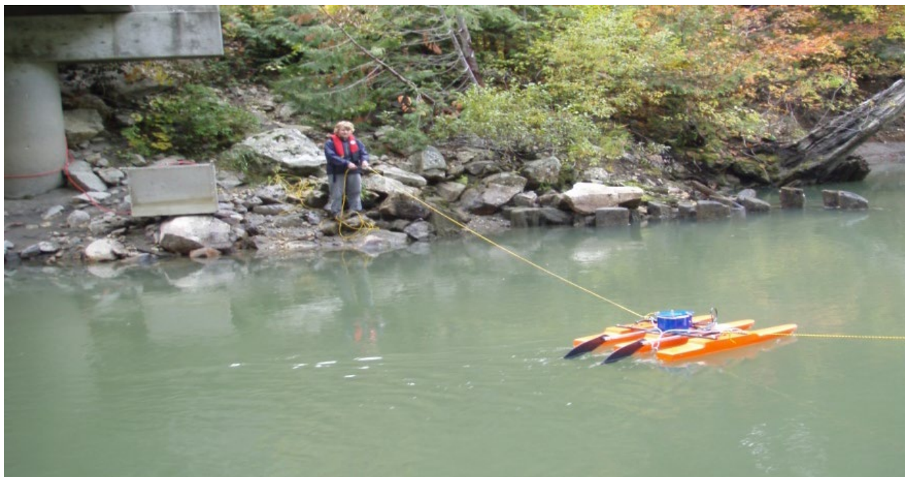
Figure A4. StreamPro raft towed from shore to shore (photo by Washington Department of Ecology).
