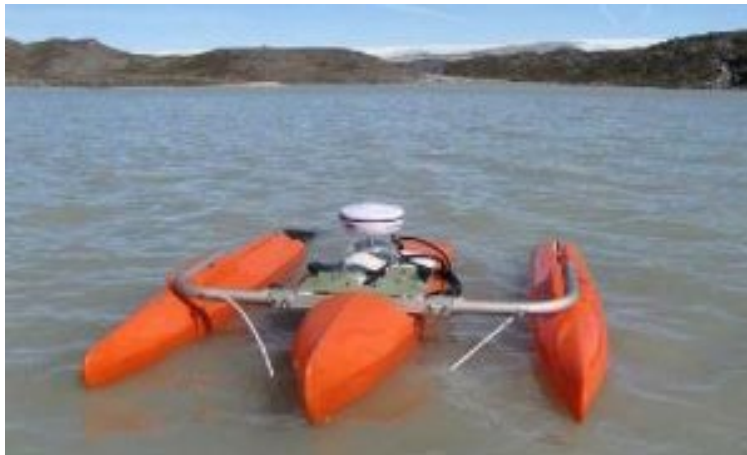
Figure 2. The three-hulled boat that houses the RiverPro head.
