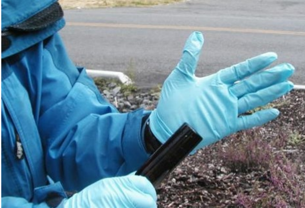
Figure 4: Checking a VOA bottle for bubbles.
