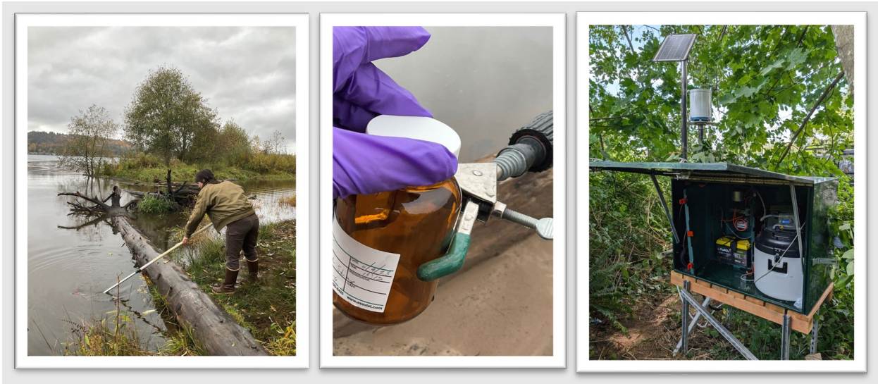
Figure 1. Left and center images are examples of grab sampling. The right image is an example of a stream station where an autosampler is set up for active sampling.
