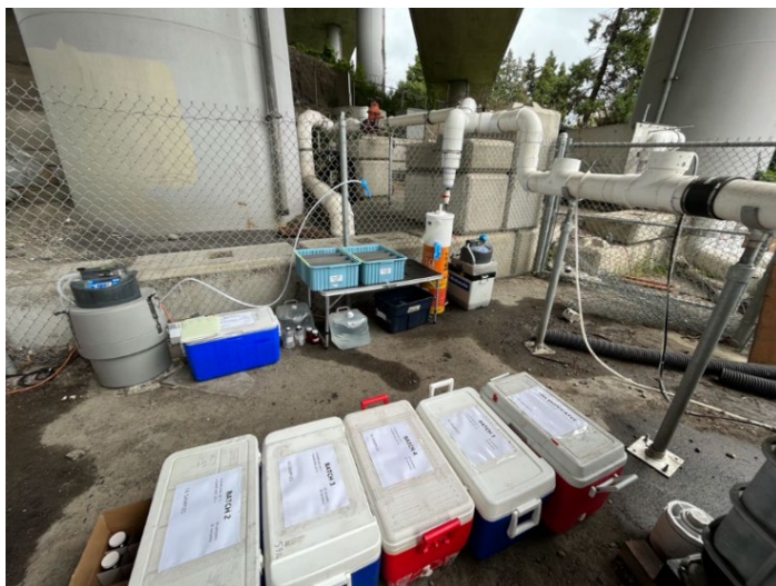
Figure 2. We want to better understand the concentrations of chemicals in stormwater when it rains, including 6PPD-q. Field staff for King County Environmental Lab collect a stormwater runoff sample from the highway above. Photo credit: KCEL.
