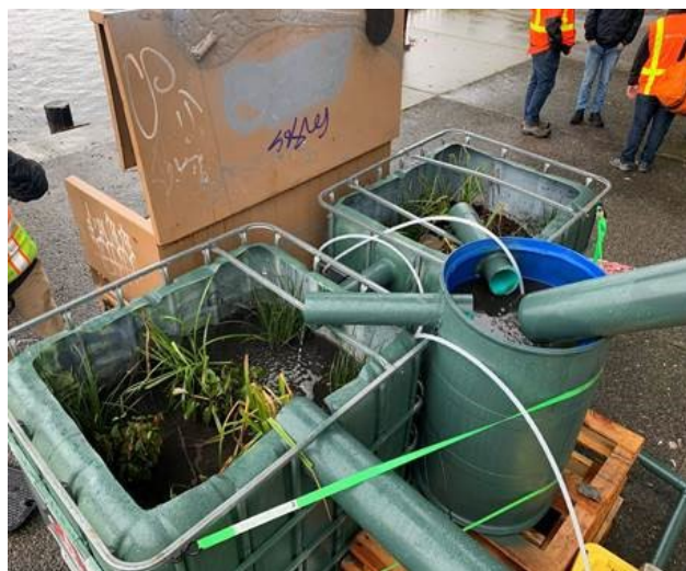
Figure 4. Stormwater retrofits help reduce 6PPD-q pollution. This pilot project tests the effectiveness of bioretention planter boxes to treat 6PPD-q. Photo credit: WSDOT.
