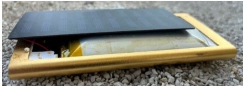
Figure 4: Lithium-ion batteries can swell when damaged or malfunctioning. In this photo, the swollen lithium-ion battery pushed on the attached solar panel, popping it out of place.
