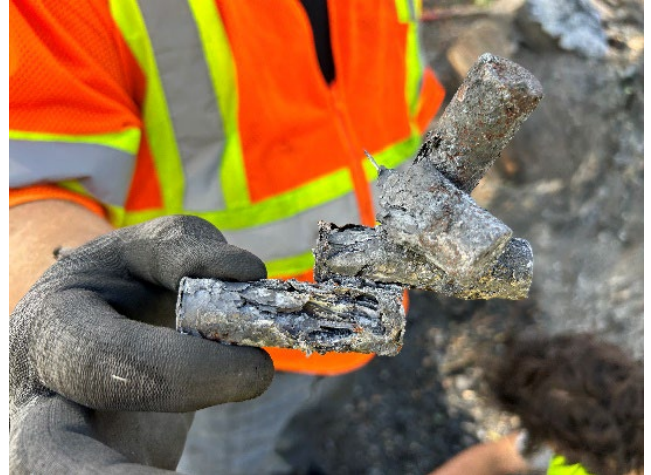
Figure 4: Electric vehicle batteries contain thousands of cells that can become severely damaged and burned during a fire.
