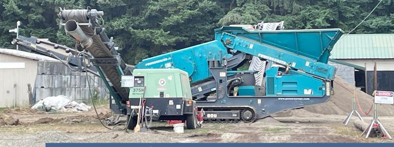
Machinery used to recover lead from impact berms. Recovered lead can be recycled.
