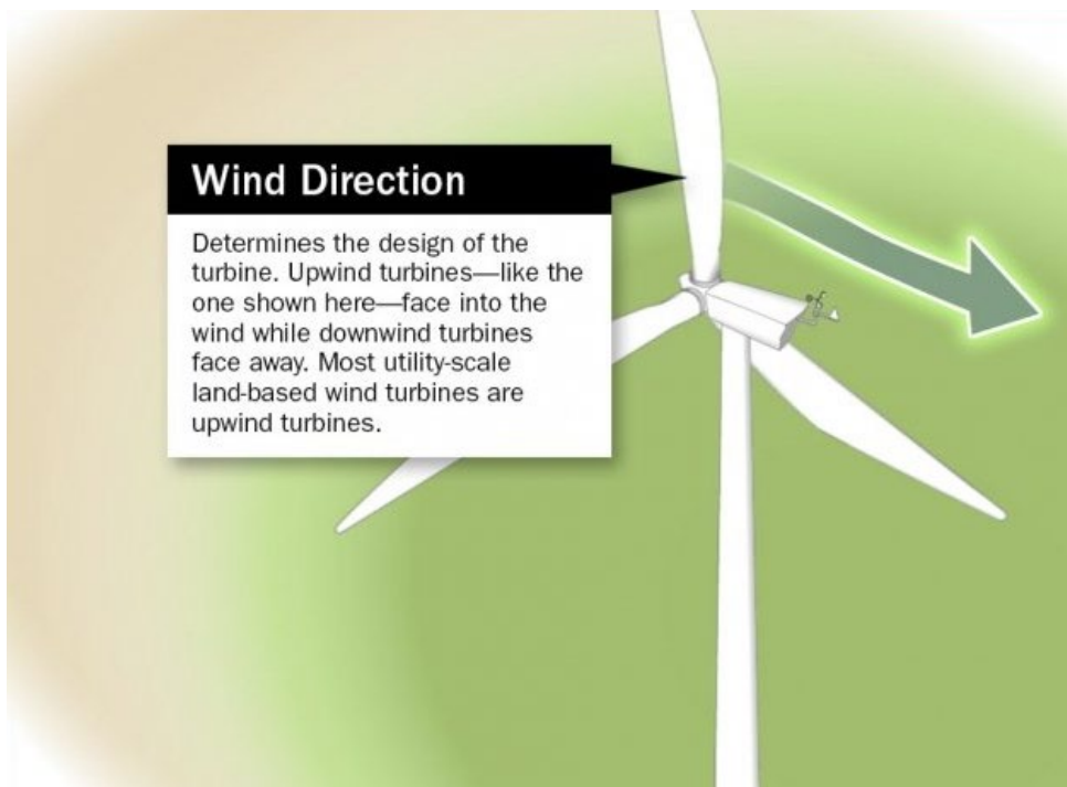
Figure 2-4. Wind turbine in upwind direction
