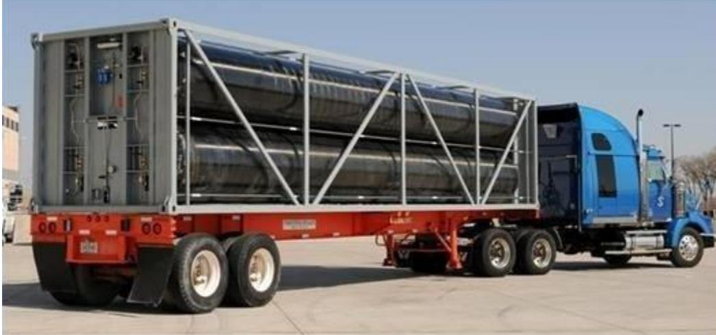
Figure 2-3. Example of a tube trailer transporting gaseous hydrogen
