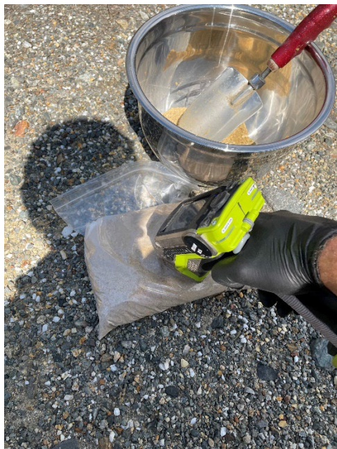
Figure 3: Conducting XRF analysis on composite sample.
