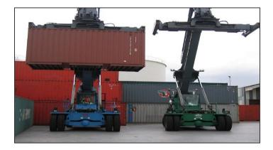
These reach stackers do the hard work of moving and stacking heavy cargo containers, so their tires have more zinc to prevent wear and ensure safety.
