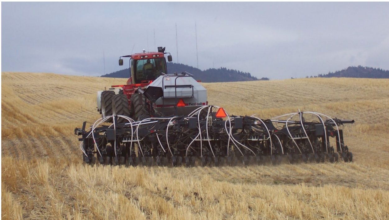
Image 3. Low disturbance direct seed drill seeding into the residue of a previous crop.
