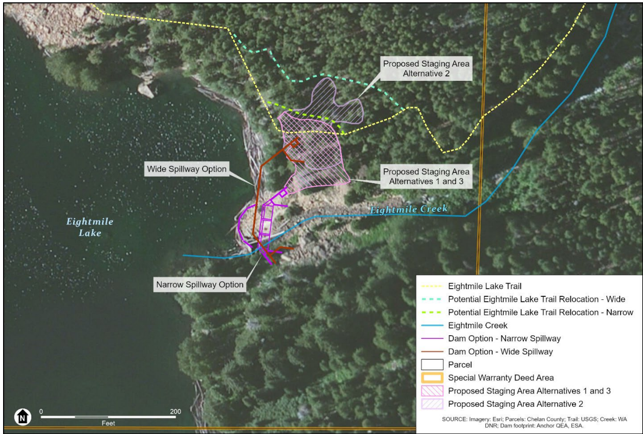
Figure 11. Dam Construction Staging Area
