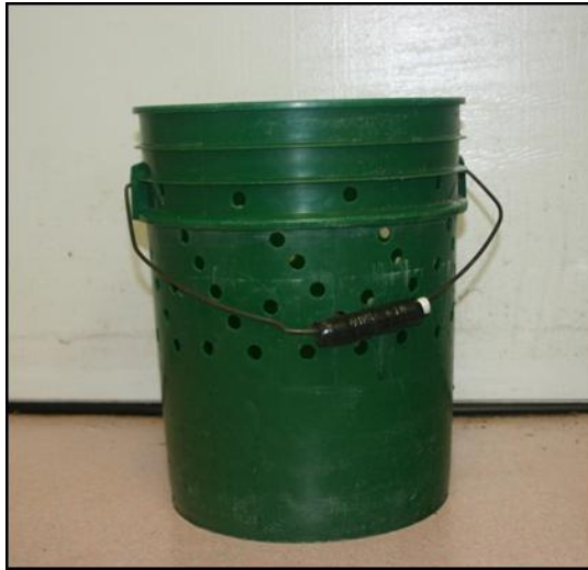
Figure 7. A perforated 19-liter recovery container. The bottom of the container is not perforated so that the reservoir holds 7-liters of water.
