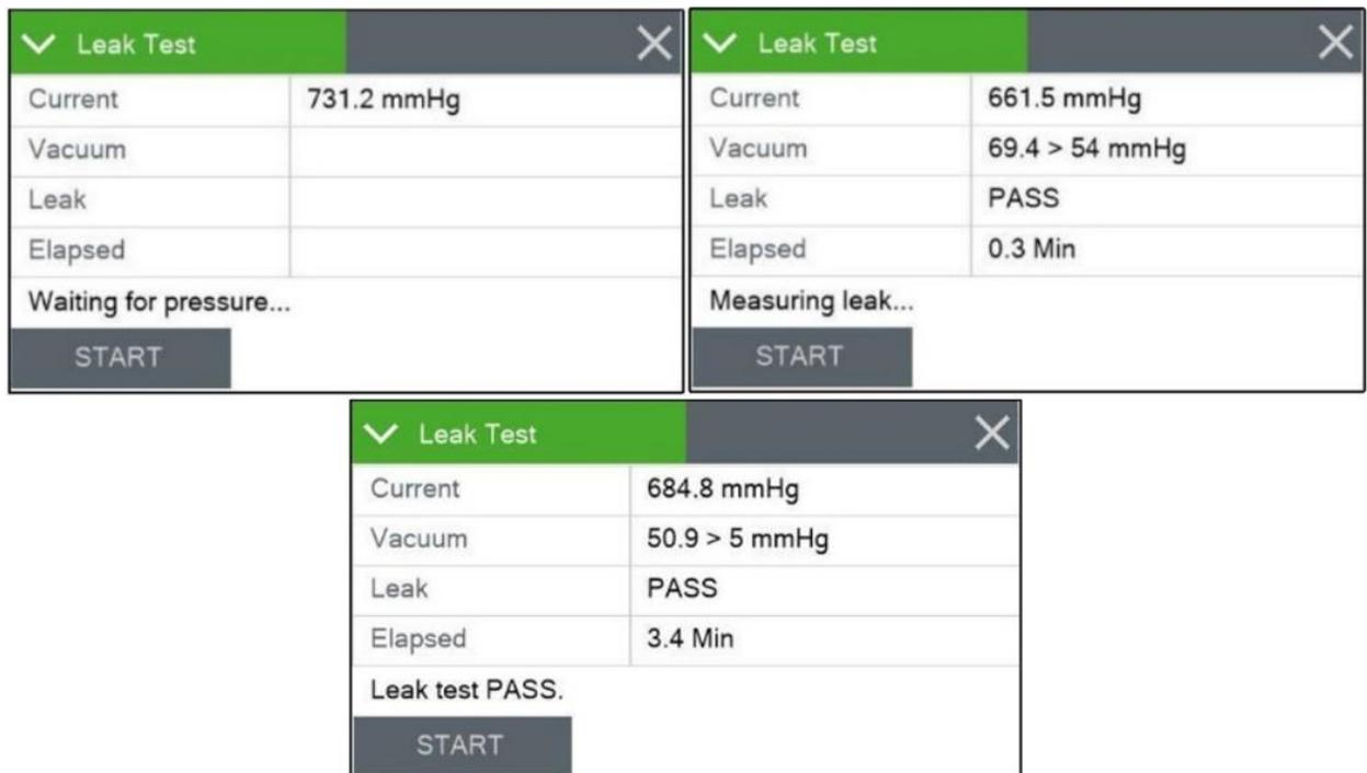
**Figure 7-3: Leak Test Result Screen (Met One, 2013)**
