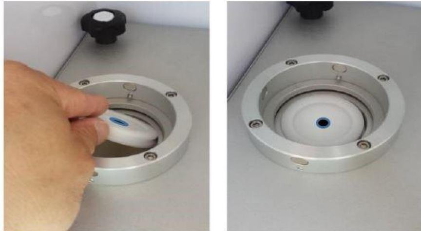
**Figure 7-2: Inserting the External Leak Test Cassette (Met One, 2013)**
