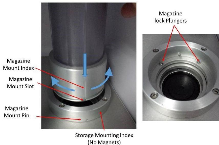
**Figure 6-7: Mounting the Storage Magazine (Met One, 2013)**
