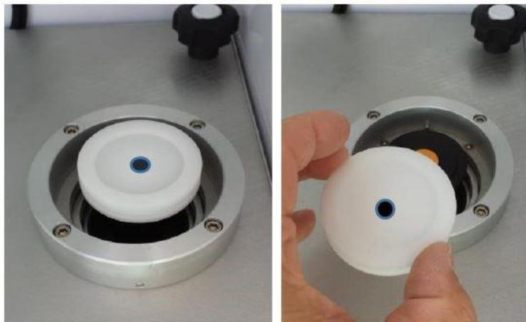
**Figure 7-5: Removing the External Leak Test Cassette (Met One, 2013)**
