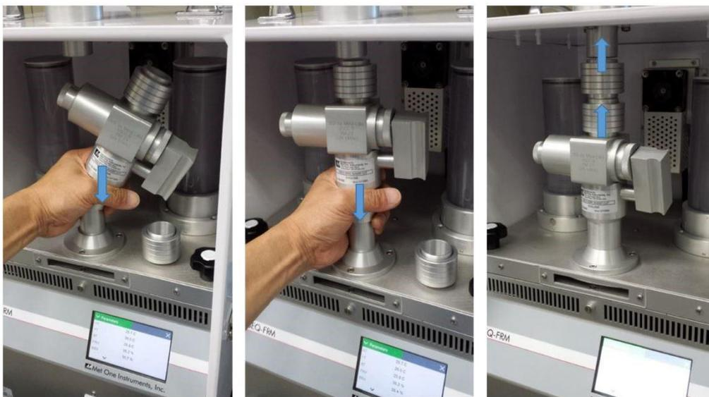
**Figure 5-2: VSCC Installation (Met One, 2013)**
