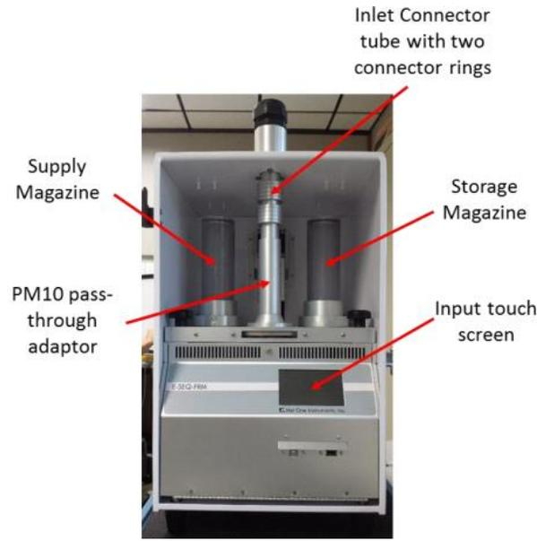
**Figure 5-1: Installation Using the PM<sub>10</sub> Pass Through Adaptor (Met One, 2013)**
