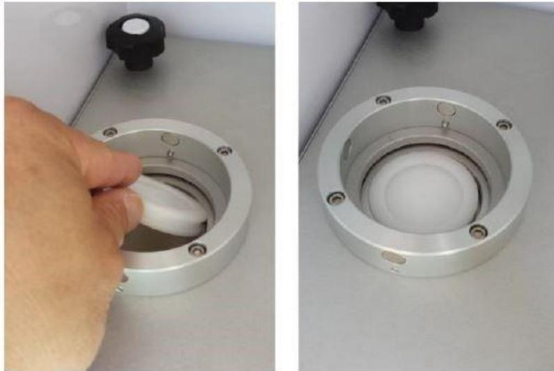
**Figure 7-6: Inserting the Internal Leak Test Cassette (Met One, 2013)**
