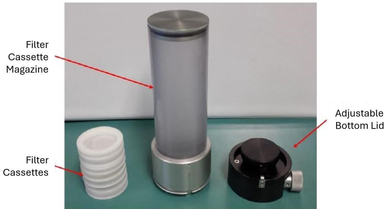
Figure 6-4: Filter Cassettes, Magazine and Adjustable Bottom Lid (Met One, 2013)
