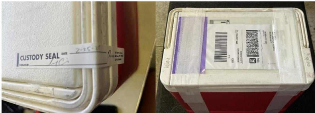
**Figure 6-9: Shipping Container with Custody Seal**
