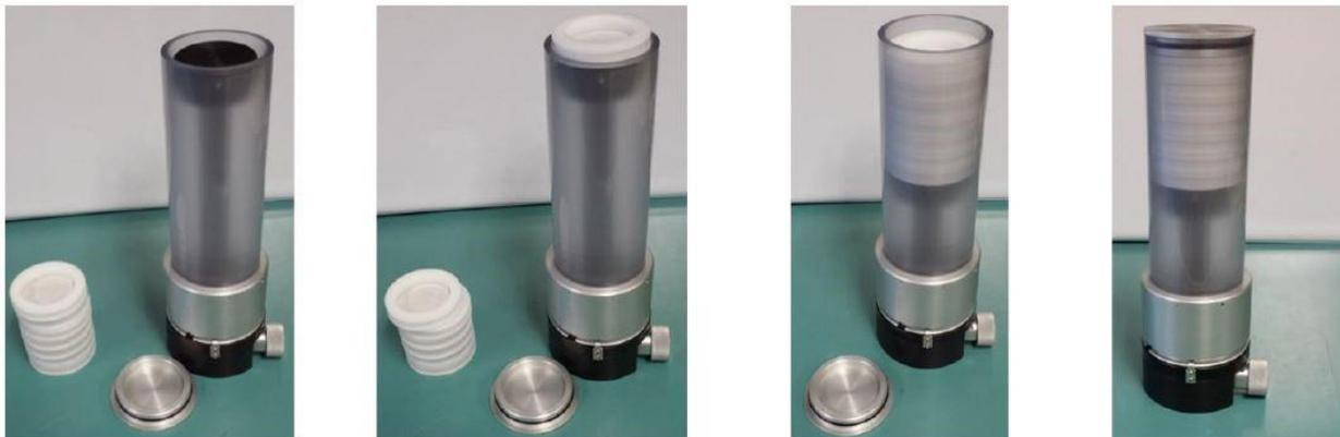
**Figure 6-6: Loading New Filter Cassettes into the Magazine (Met One, 2013)**
