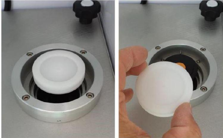
**Figure 7-7: Removing the Internal Leak Test Cassette (Met One, 2013)**
