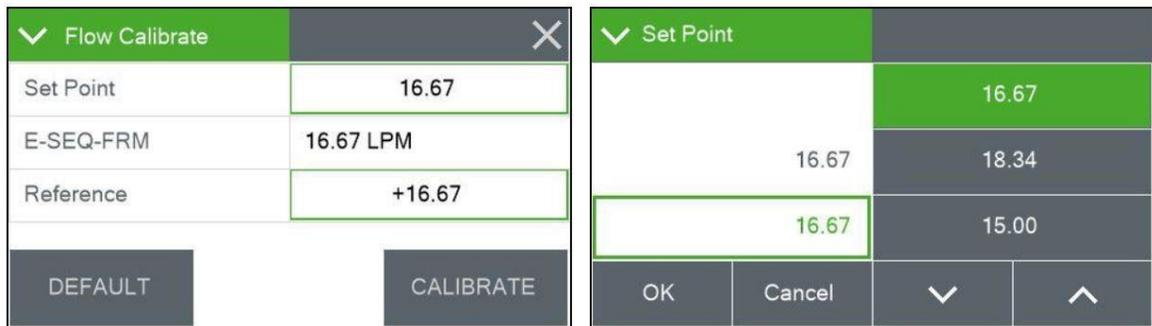
**Figure 7-16: Flow Calibration Flow Rate Selection Screen (Met One, 2013)**
