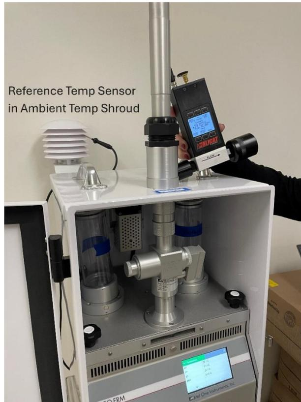
**Figure 7-8: Ambient Temperature Sensor Audit**
