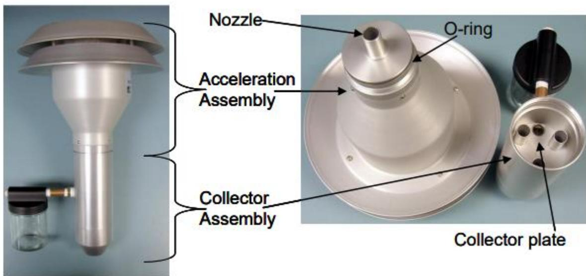
**Figure 7-13: Diagram of PM<sub>10</sub> head inlet components (Vaughn, 2009)**
