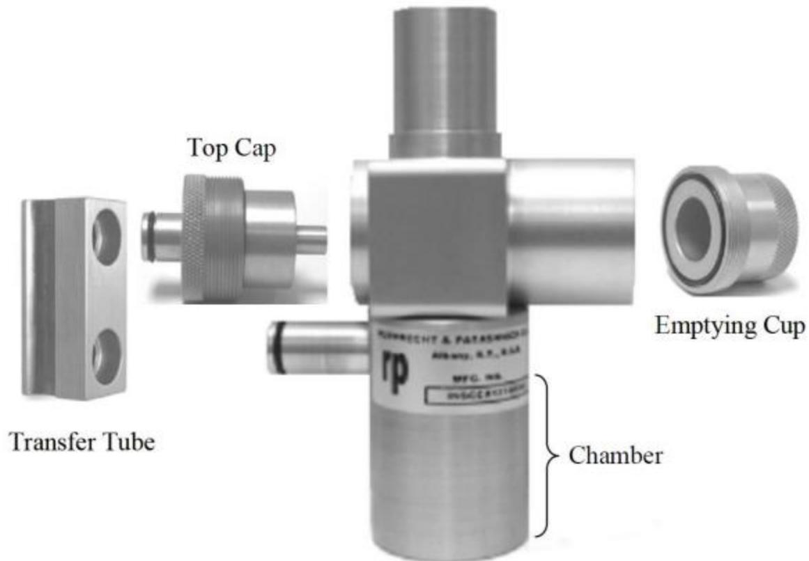
Figure 7-14: Exploded view of VSCC components (Vaughn, 2009)
