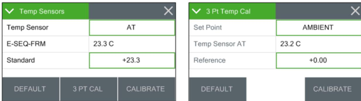
Figure 7-17: Temperature Calibration Screens (Met One, 2013)
