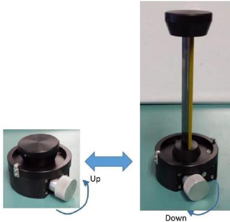
**Figure 6-5: Adjustable Bottom Lid Operation (Met One, 2013)**
