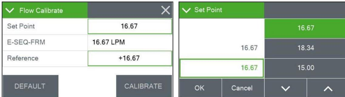
**Figure 7-12: Flow Calibration Flow Rate Selection Screen (Met One, 2013)**
