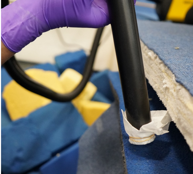
Figure 10. Floor dust sample collection using a vacuum wand extension fitted with a Kimwipe.
