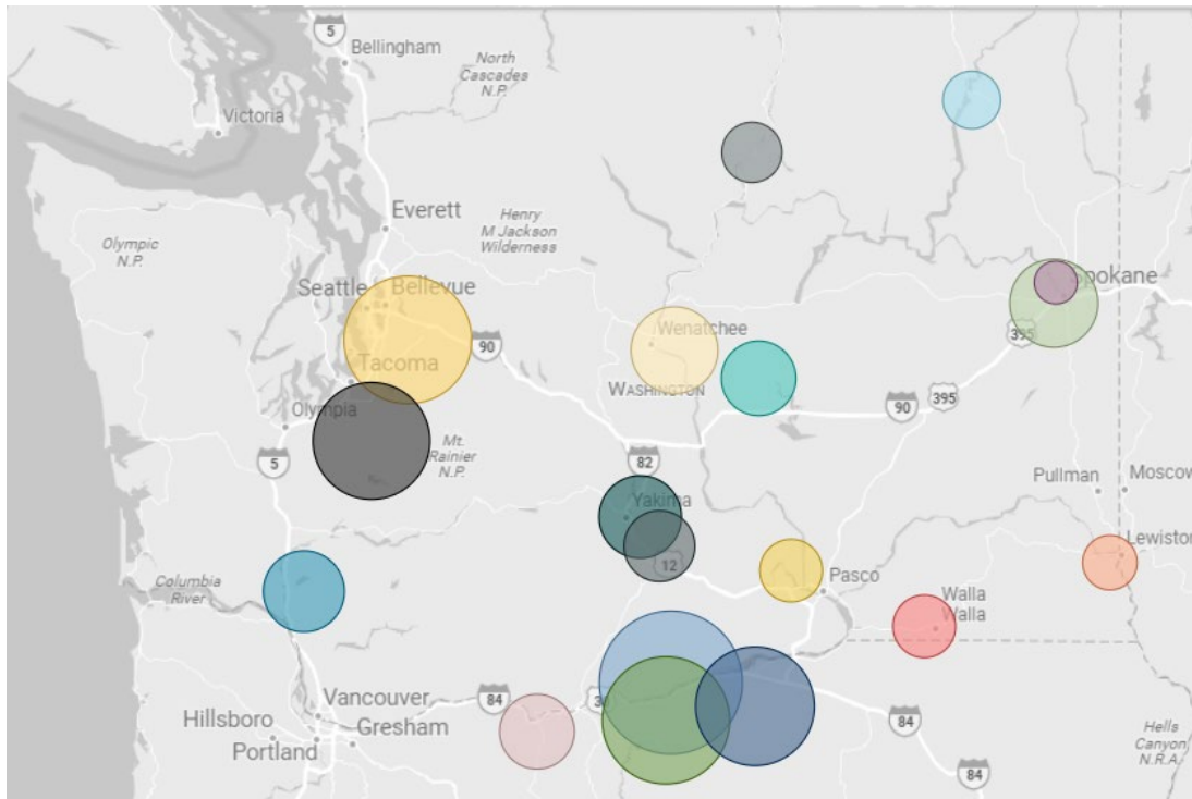
Figure 2 Municipal solid waste disposal facilities that take solid waste generated in Washington State. The size of the dot represents the amount of solid waste disposed at the facility, with most waste being sent to facilities in central Puget Sound or south central Washington.
