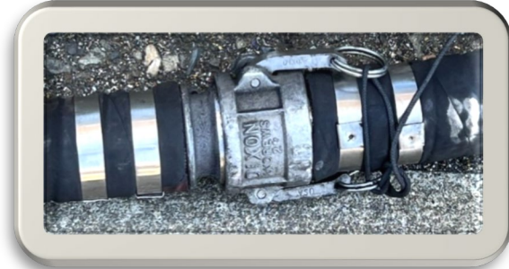
A camlock connection with cam arms secured with twine.
