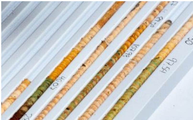
Figure A2. Bromocresol green stained sapwood in several Douglas-fir core samples.
