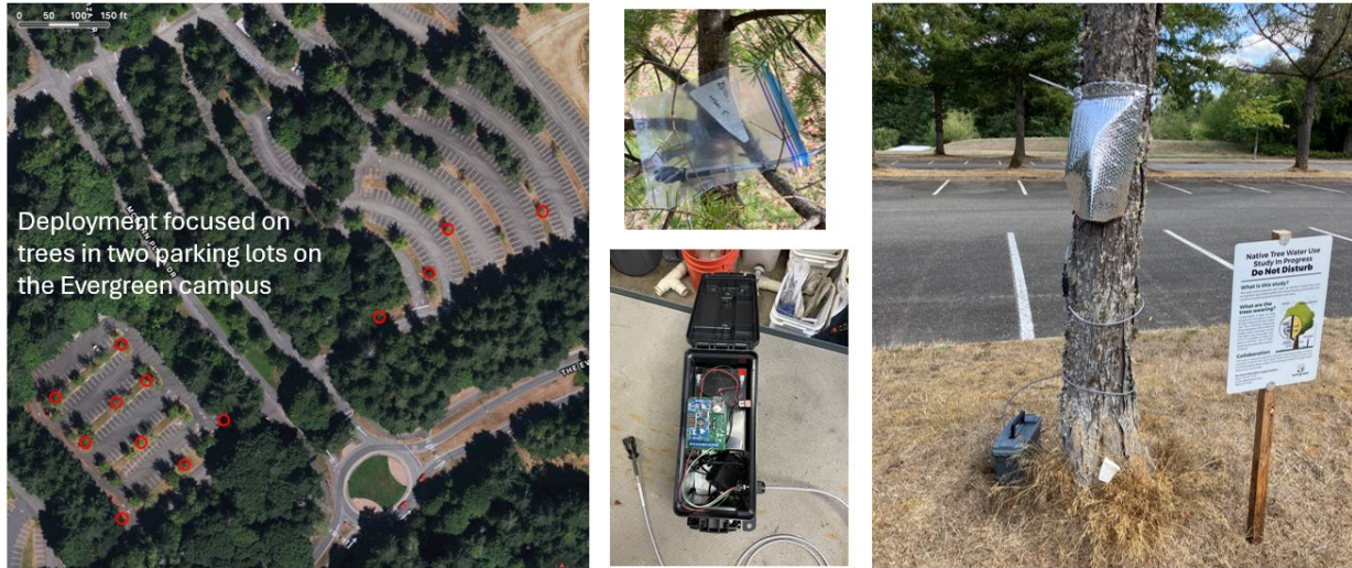
Figure 13. Details on mobile probes. Washington State University (WSU) and TESC developed and deployed a mobile data logger (smaller and cheaper than the traditional approach) at twenty street tree locations in 2023 and 2024. These mobile data loggers are deployed for 2-3 days at a time, and the 2 nd or third day is used for sap flux data (allowing the first day for equilibration of the heated probe to the tree).
