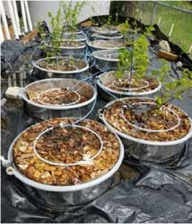
Figure 1. Six experimental bioretention soil mesocosms in 55-gallon drums received stormwater collected from Interstate-5 highway.
