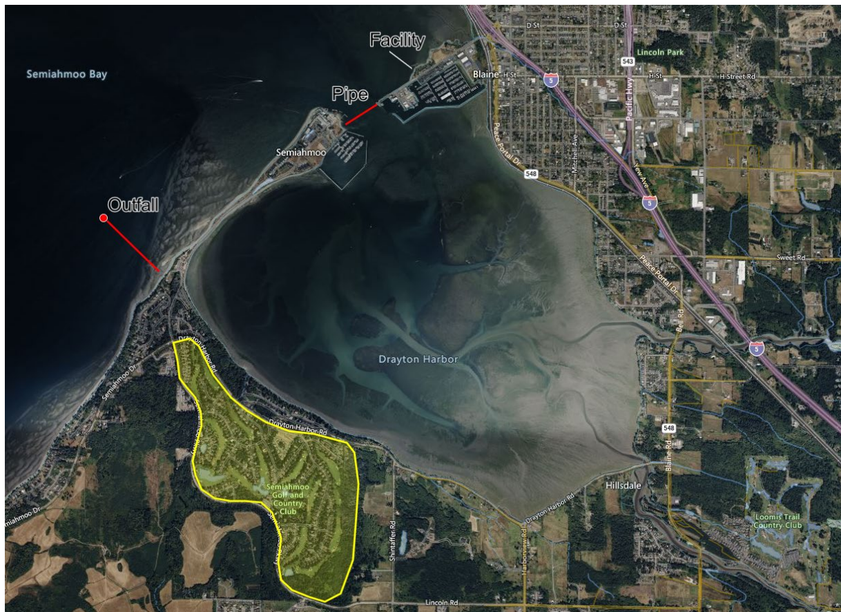
Figure 11. Lighthouse Point Water Reclamation Facility location, two submarine pipes crossing the mouth of the harbor, outfall 001, and reclaimed water use area (outlined in yellow)
