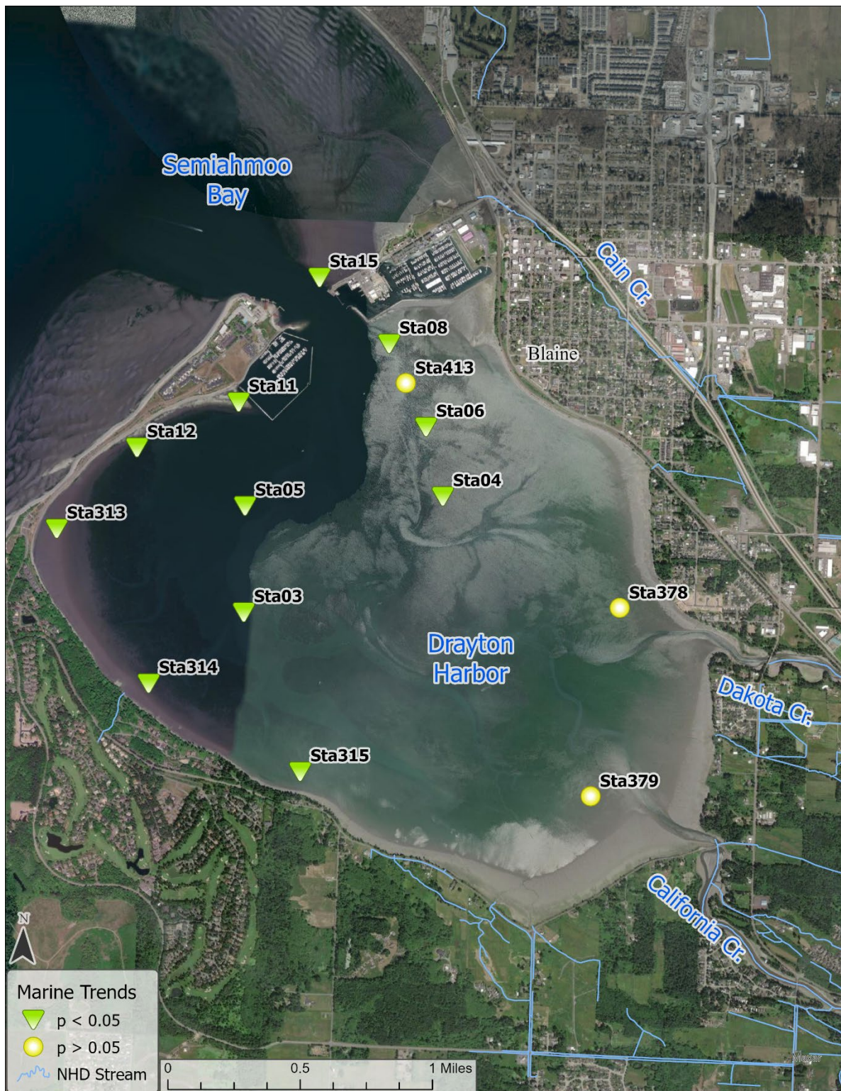
Figure D-69. Fecal coliform (FC) concentration trends at the DOH marine monitoring stations in Drayton Harbor where p < 0.05 = strong improving trend indication, 0.05 < p < 0.1 = weak trend indication
