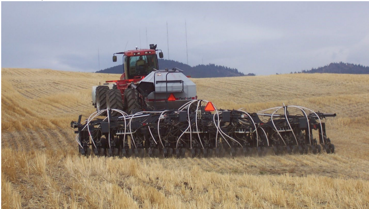
Figure 26. Low disturbance direct seed drill seeding into the residue of a previous crop
