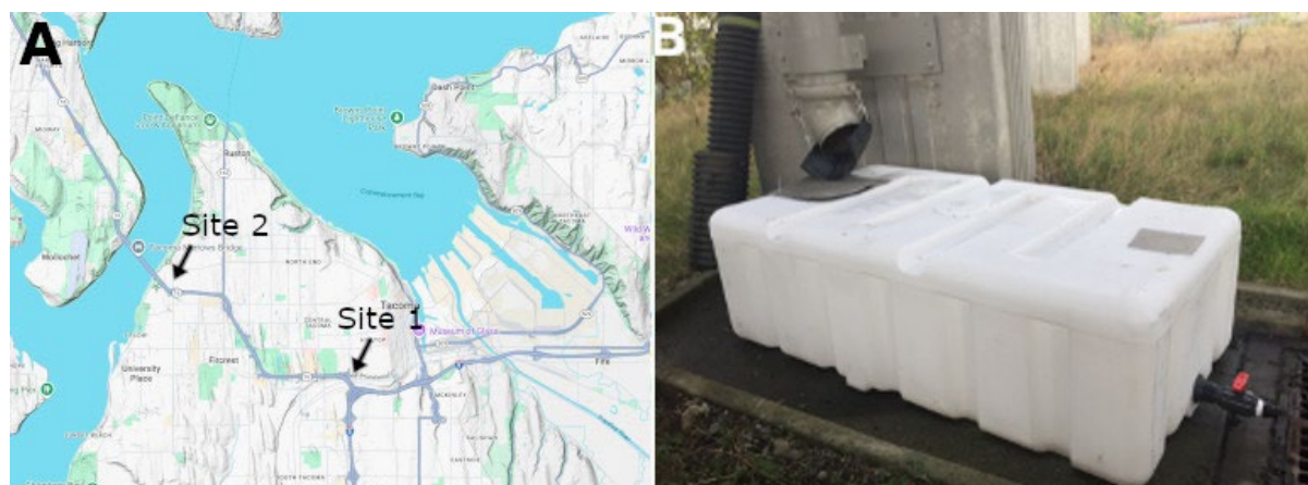
Figure 3. Stormwater runoff collection sites. A) Approximate collection sites on west-bound SR16. Site 1 was used for Events 1-57 (47° 14' 4.47" N, 122° 27' 48.05" W). Site 2 was used for Events 58-78 (47° 15' 48.98" N, 122° 32' 38.89" W). B) 500-gallon polyethylene collection tank used to collect urban stormwater runoff.
