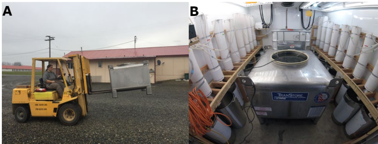
Figure 5. Stormwater runoff transportation. A) Transportation tanks filled with stormwater runoff are moved into the temperature-controlled chamber. B) The clean water tank (rear) and stormwater transportation tank (front) in the temperature-controlled chamber with the experimental bioretention modules.
