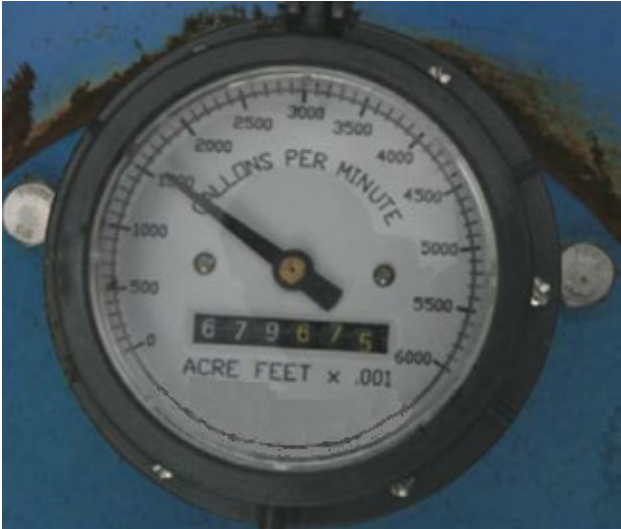
Figure 4. This meter has a flow rate indicator, reading in gallons per minute. The totalizer reads in acre-feet x 0.001. The reading on the meter is 679,675 acre-feet x 0.001, or 679.675 acre-feet.
