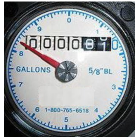
Figure 2. Meter face with a fixed totalizer number and a sweep hand.
