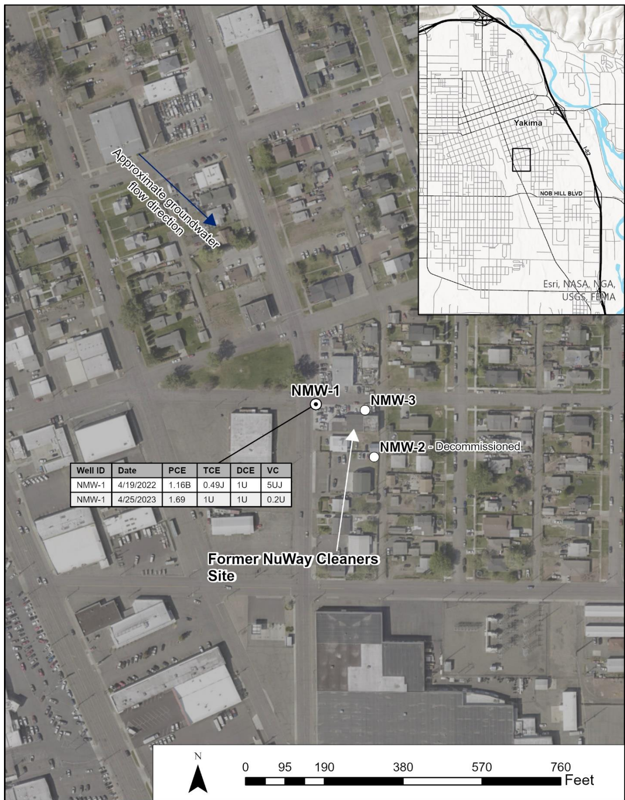
Figure 4. Nu-Way Cleaners well locations and cVOC results ( \mu\text{g/L} ), 2022 – 2023.
