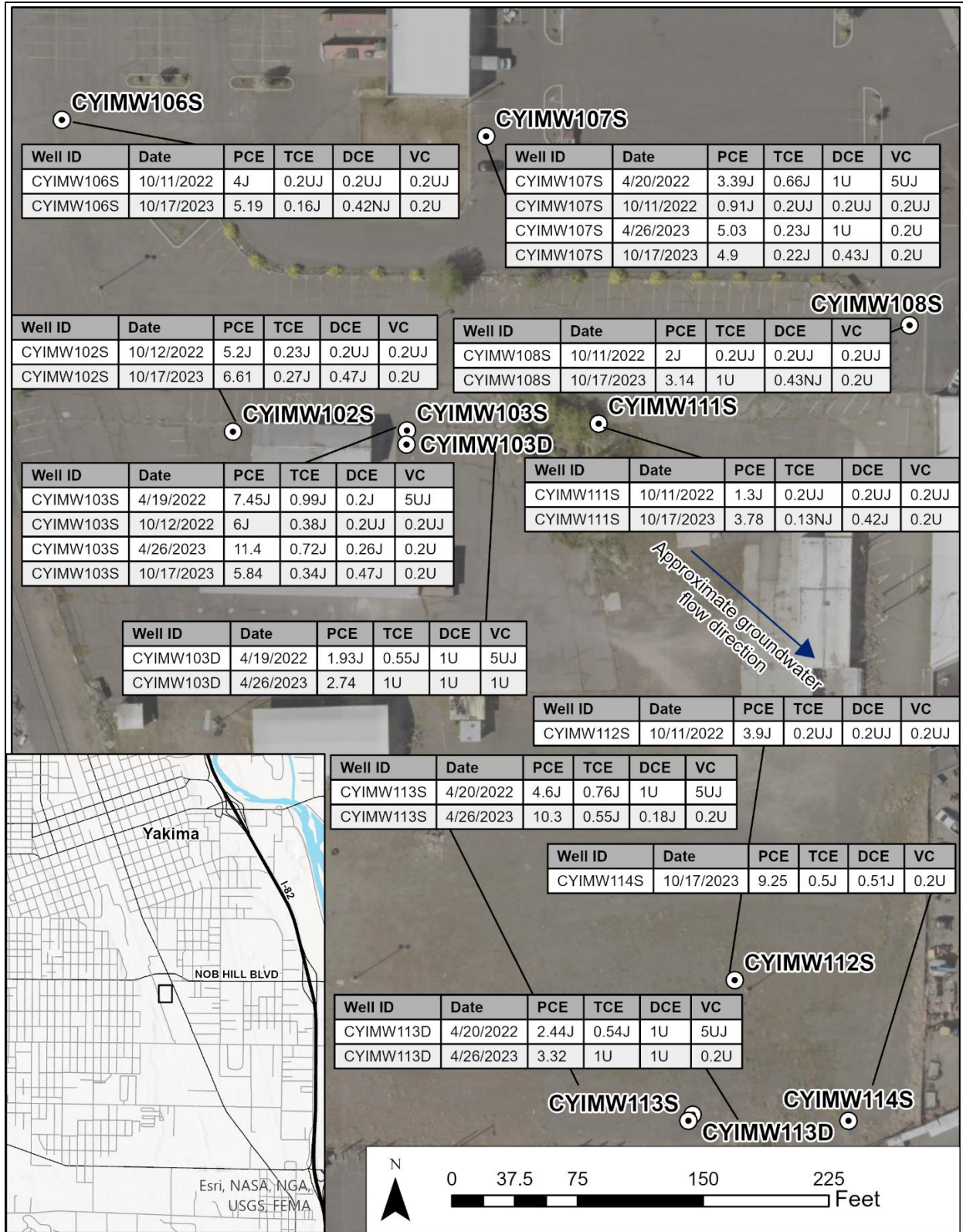
Figure 7. Cameron Yakima well locations and cVOC results ( \mu\text{g/L} ), 2022 – 2023.
