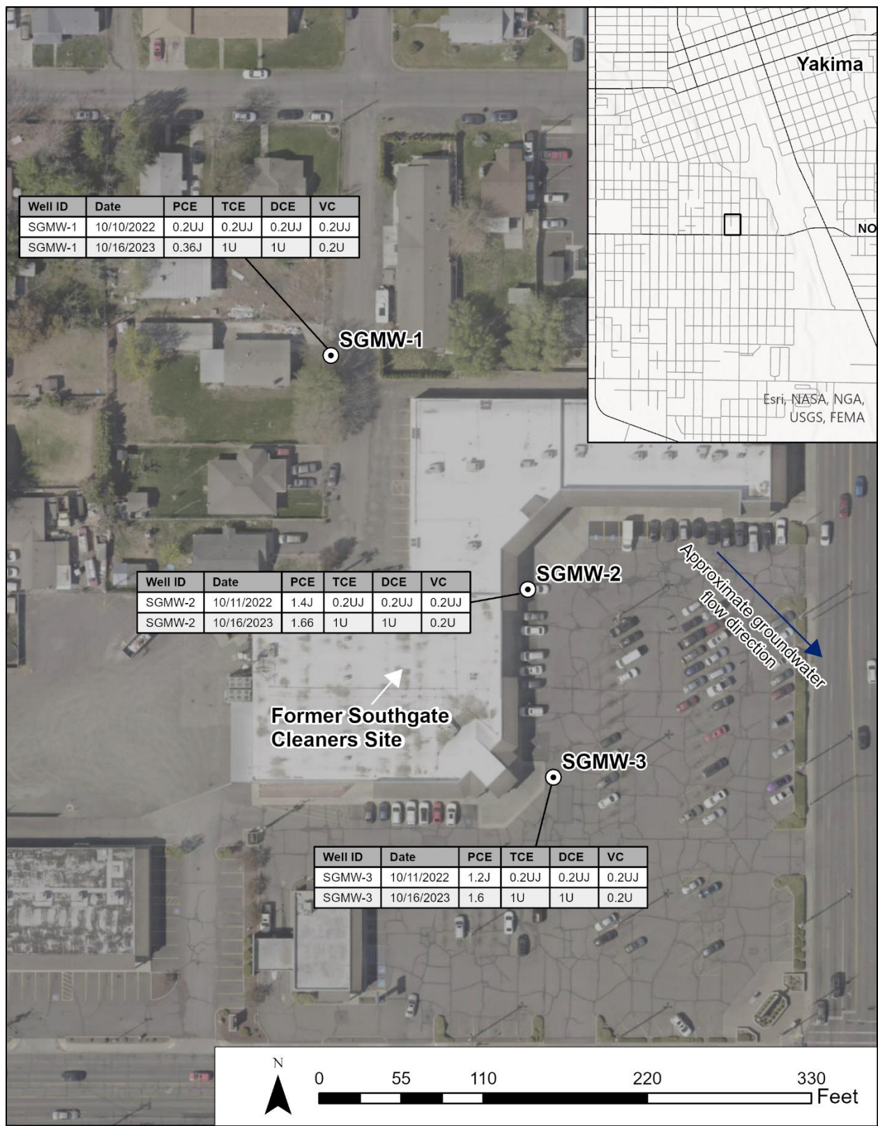
Figure 5. Southgate Laundry well locations and cVOC results ( \mu\text{g/L} ), 2022 – 2023.
