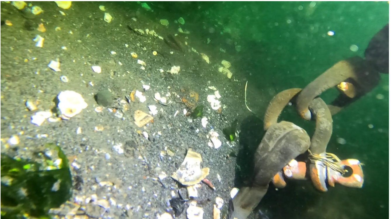
Buoy 3: Anchor eye, shackle, and swivel in good condition.
