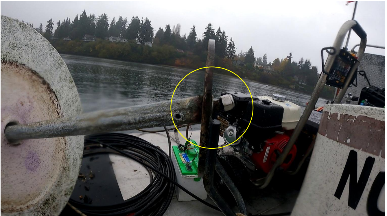
Buoy 2: Can removed. Threads bent likely from vessel impact
