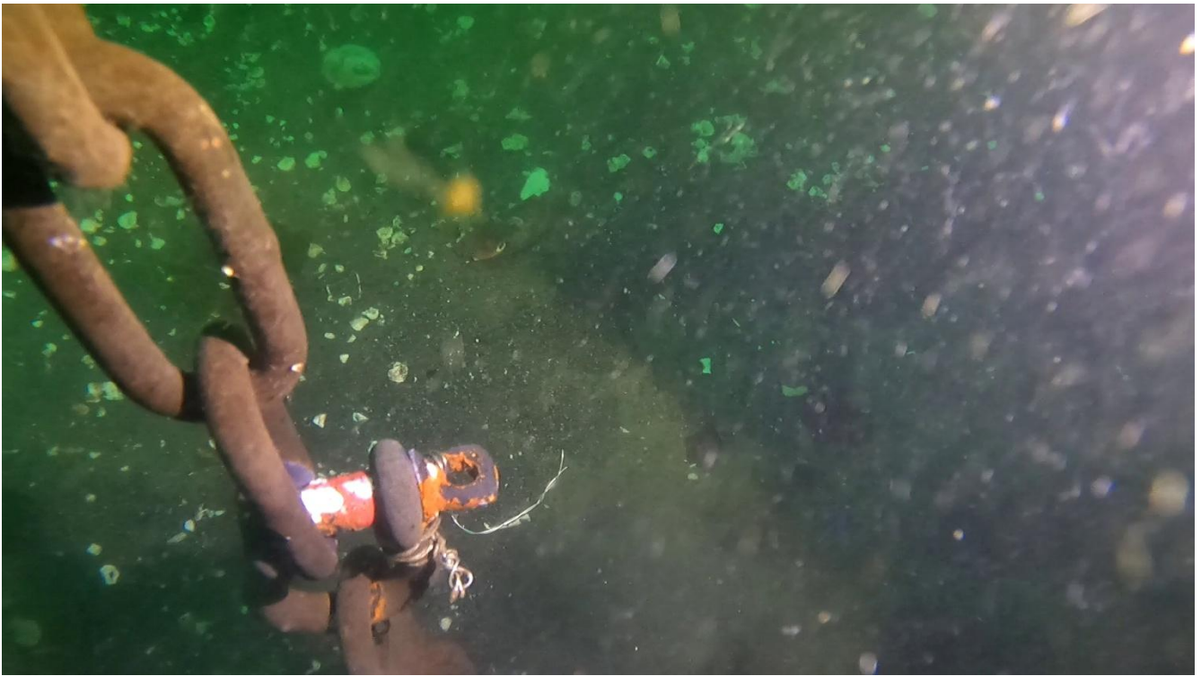
Buoy 3: Typical Anchor shackle and lower chain condition. Galvanizing intact, lower section of chain in good condition.
