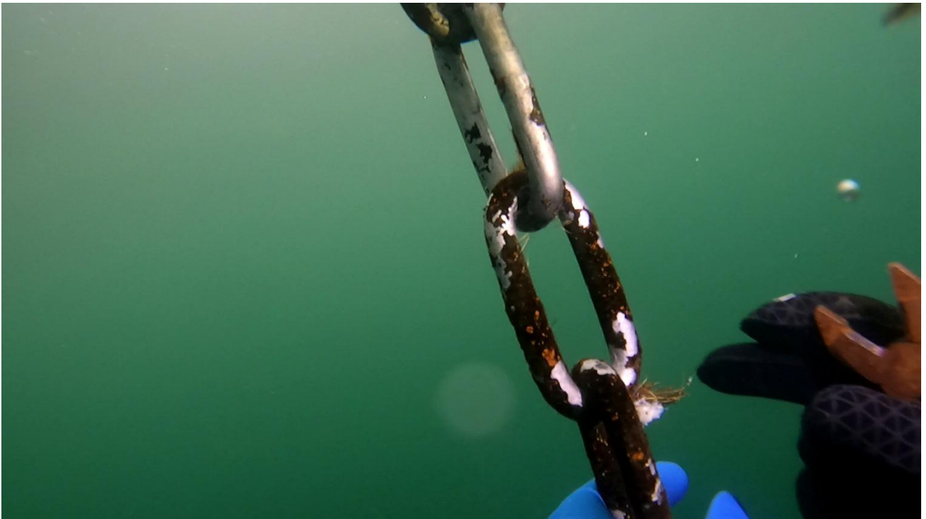
Buoy 2: Typical chain condition
