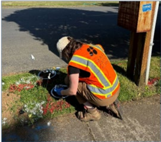
Figure 20: 2025 Right-of-Way Sampling to Determine Depth of Excavation
