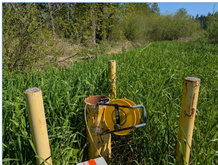
Figure 11: Post permeable barrier wall installation groundwater sampling at well on B&L Woodwaste landfill.
