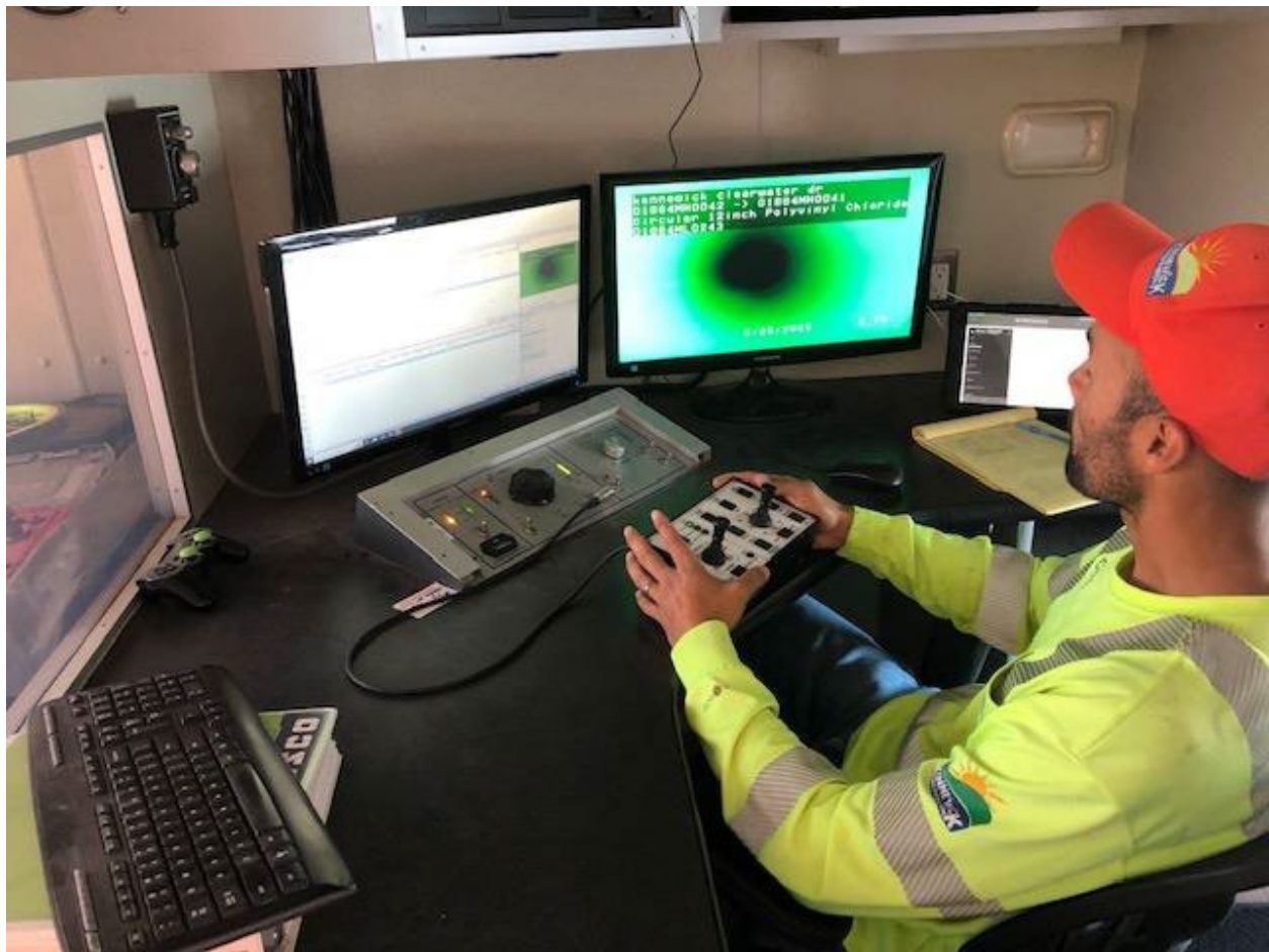
25 New inspection equipment helps Kennewick identify stormwater system issues and meet permit requirements. Photo by: City of Kennewick.
