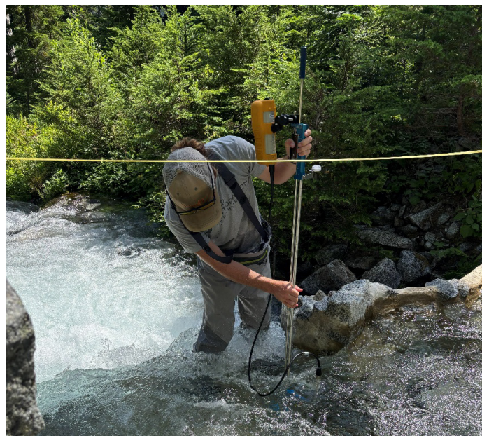
Photo: FlowTracker2 Monitoring Setup
