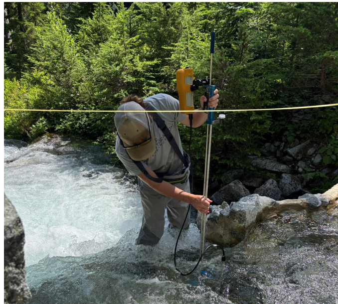
Figure 3. FlowTracker2 Monitoring Setup
