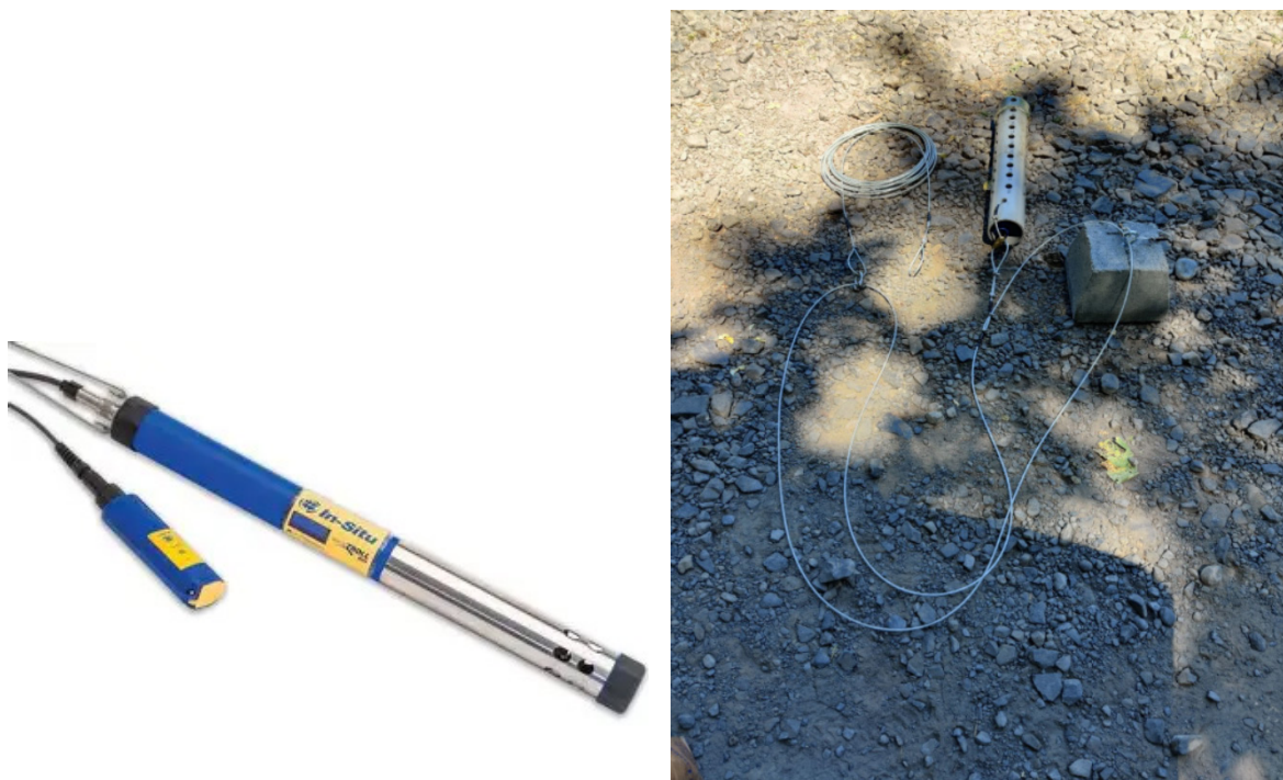
Figure 7. In-Situ Aqua TROLL 600 Water Quality Sonde and an Example Deployment System for Monitoring Dye Concentration.
