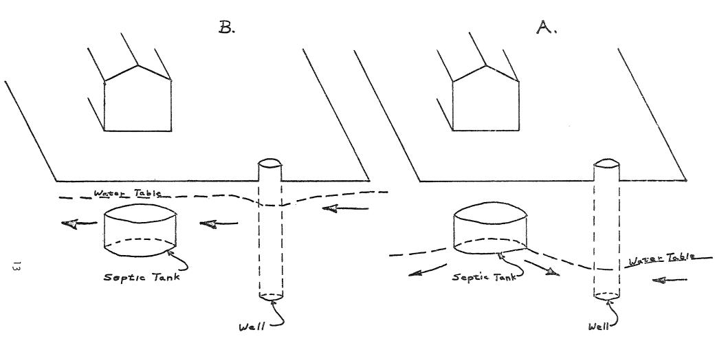
Arrows indicate direction of ground water flow.
