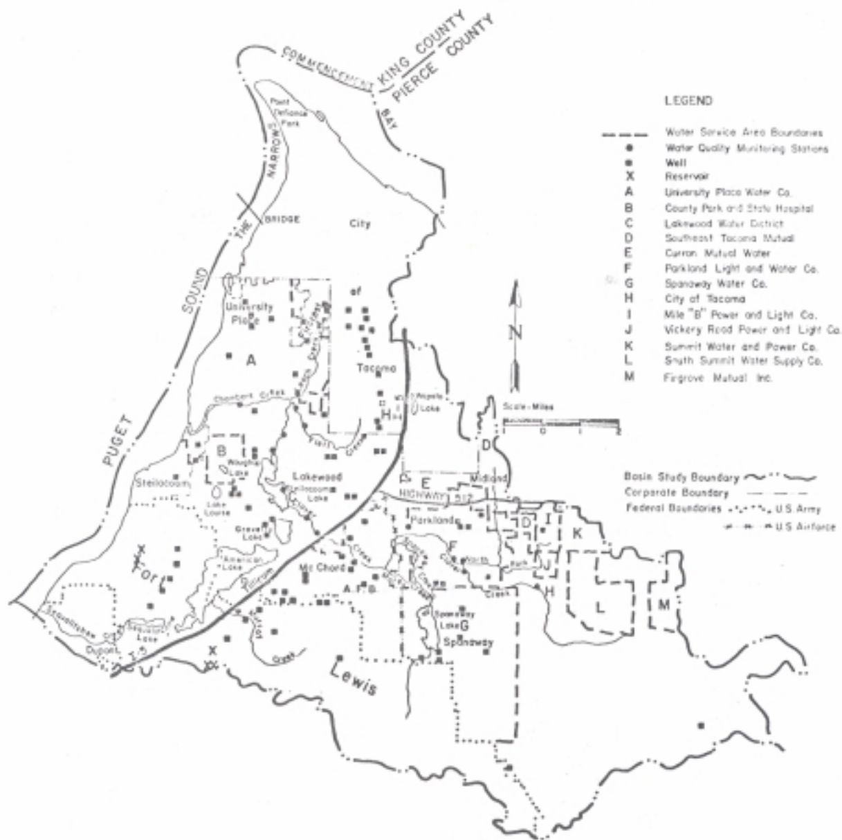
FIGURE 2. Chambers-Clover Creeks Basin (WRIA-12). Map indicates locations of special water districts, water companies, wells, reservoirs, and water quality monitoring stations. (Modified from Kennedy Engineers, Inc., 1974)
