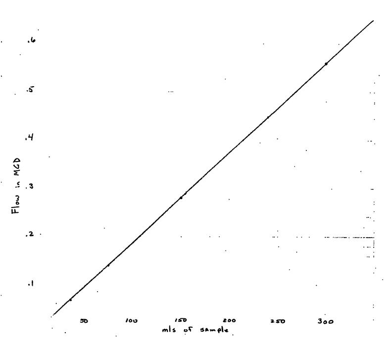
Figure 1. Sample graph for calculation of flow proportional composite. Based on maximum flow of .56 MGD.
