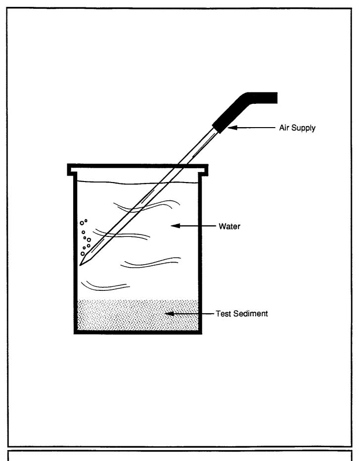
Figure 1. Static exposure system used for the *Neanthes* sublethal bioassay
