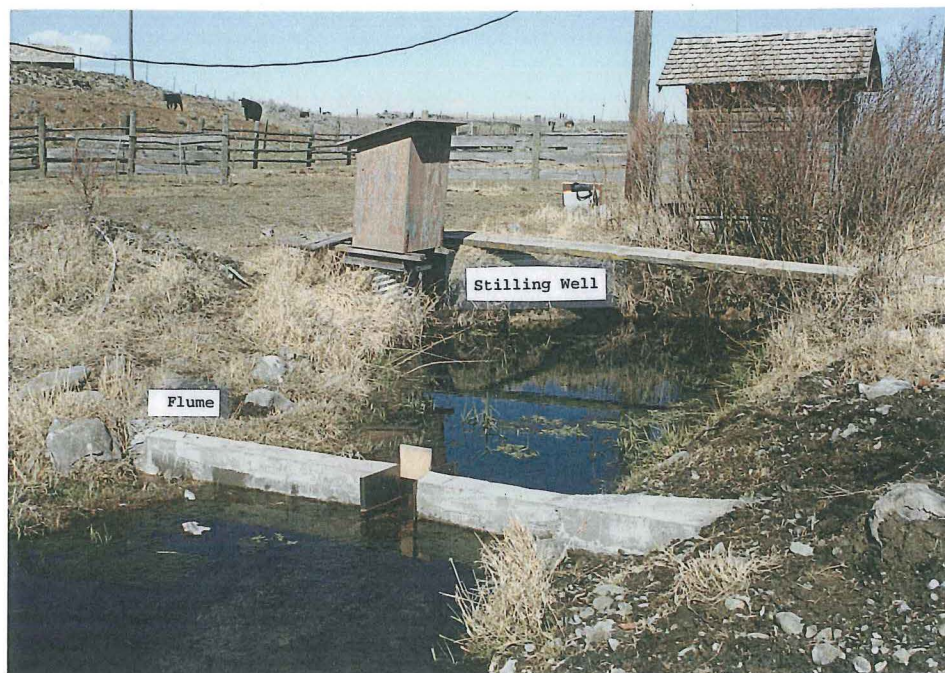
Plate 1b. Close-up of Baring Spring. Basalt outcrop can be seen along the top left edge of the picture. Continuous monitoring equipment was stored within the enclosure attached to the top of the stilling well.
