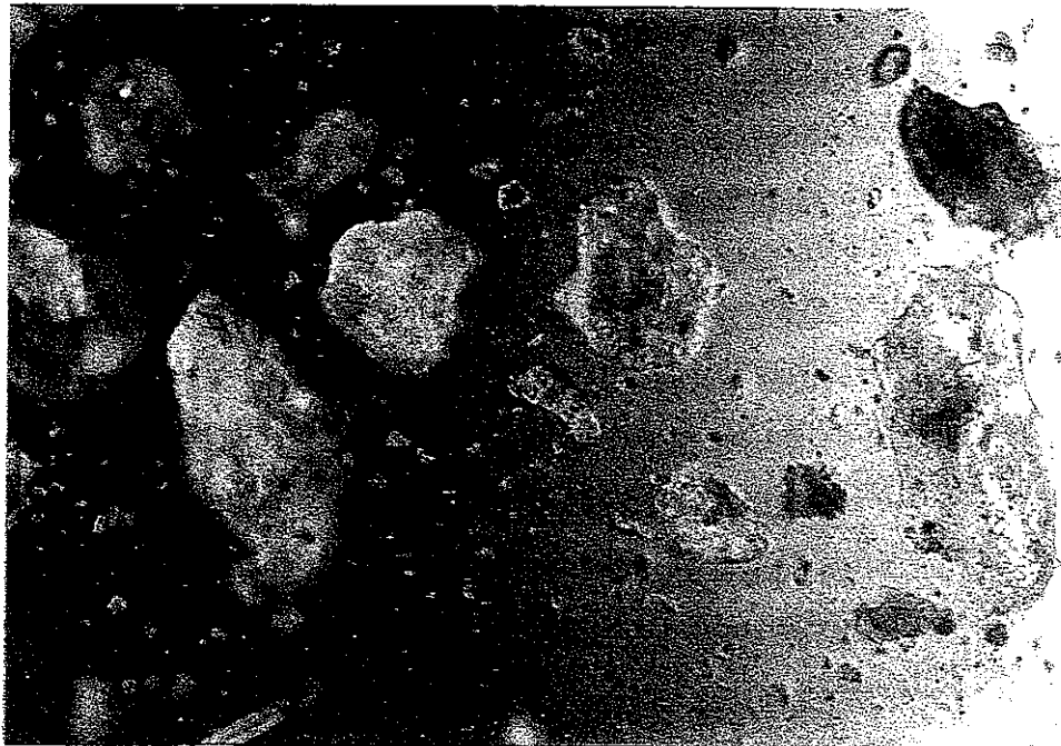
Figure 12. Station RC-2, Sample 96378295, 100X oblique illumination. Note orange-yellow coating in transparent mineral grains.
