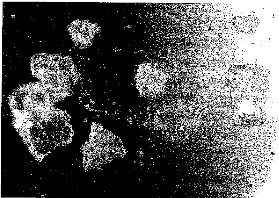
Figure 9. Tailing pile TP-2, Sample 96378322, 100X oblique light. Note the orange-yellow coating on the clear mineral grains.
