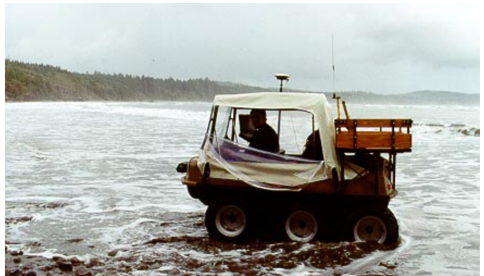
An amphibious vehicle rigged with Global Positioning System equipment maps the beach at Point Grenville as part of the Southwest Washington Coastal Erosion Study.
